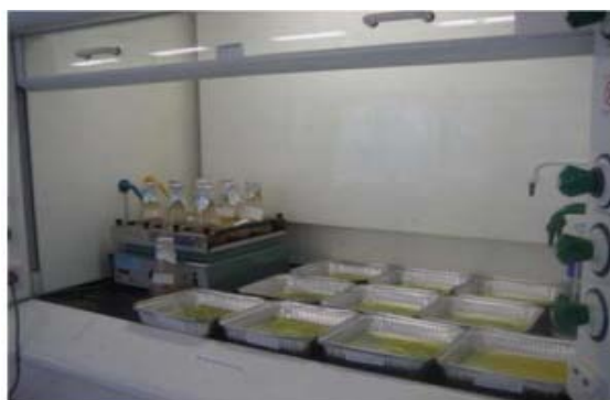
Fig. 2: Chemical oil extraction using n-hexane [23]
