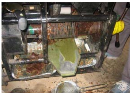
Fig. 1: Mechanical oil extraction through a screw press [23]
